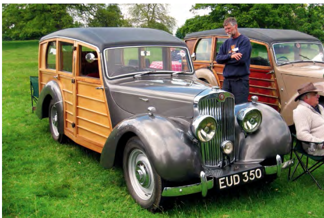
The Lea-Francis 14hp became a favourite for conversion into a shooting brake in the late 1940s, built first by companies including Jensen Motors and the Southern Caravan Company, before work was moved to Lea-Francis' main body supplier, APA
