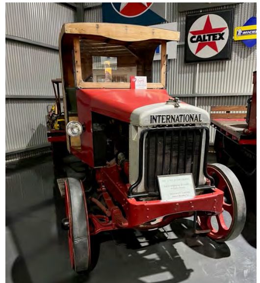
1926 International truck Hard rubber solid non-pneumatic tyres
