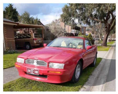
Chassis no 2. 5.3 litre V8 330 BHP. 3 Speed Auto [Chrysler] gearbox. Alloy Body, last hand built Aston ,before Steel body DB7. 355 of our model & 1050 total varieties over 6 years. Ford [ owners of AM ] built 7,500 DB7s. AM used lots of other car parts in their cars & DB 7 was Jaguar based.
