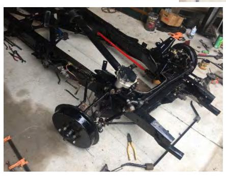
I now have a rolling chassis with all brake lines fitted and new hoses on order and the only things left to do in this area is new shockers at the front and fit the refurbished ones in the rear plus fit the anti roll bar with new rubbers.
