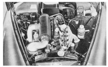
Although the six-cylinder 2.6-litre engine takes up a fair amount of room under the bonnet, components needing routine-checking are easily reached. As seen here, the brake fluid reservoir (o/s bulkhead), coil and oil filler (behind radiator), ignition distributor (above exhaust manifold) and sparking plugs can be reached without trouble. Air for the two horizontal S.U. carburettors is drawn via an oil-bath cleaner and separate silencer.
