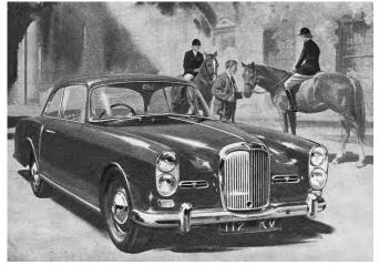
air intakes break up the otherwise plain and extensive panels between the new lamp clusters and the traditional grille. An improvement has been made to the appearance at the back by turning-under the lower edges of the wing valances
