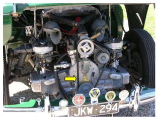
Virtually every British classic car has, hidden away under the bonnet, a drive belt. Such belts are usually of the V-section type, often referred to as 'wedge-section' belts. This is because the drive loads are transmitted via the wedging action of the belt to the grooves in the various pulleys.
