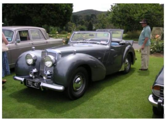
The beautiful Triumph 1800 Roadster owned by Paul and Maggie Brooks, see inside for details of this fine motor car was brought back to life. These fine cars had many attributes, such as a tubular steel chassis and a body formed from aluminium supported on a wooden frame. The front mudguards were steel, no doubt to save the cost of under-guards to prevent the dreaded stone pimples syndrome.
